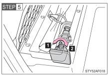
Loosen and remove the jack.
