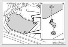
Secure the front floor mat using the hooks provided.
