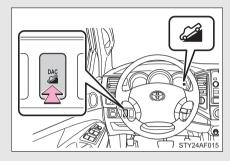
Press the DAC switch. The indicator will come on, and the system will operate.
