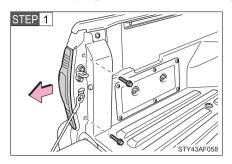
Remove the bolts and rear combination assembly.
