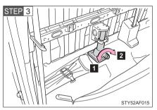
Loosen and remove the jack.
