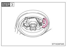
Release the bulb retaining spring.
