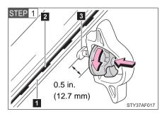
Loosen the thumb wheel in a counterclockwise motion, and depress the wheel so that the locking plate maintains 0.5 in. (12.7 mm) gap.
