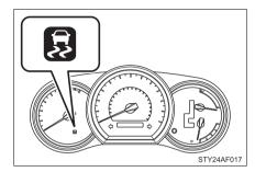
If the vehicle is in danger of slipping, the rear wheels (2WD modor four wheels (4WD models) spin, the vehicle starts to roll backwards when starting incline. this indicator on an flashes to indicate that the VSC/ TRAC/hill-start assist control systems have been engaged.
