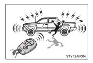
When hold is pushed for longer than about one second, an alarm will sound for about 60 seconds and the vehicle lights will flash to deter any person from trying to break into or damage your vehicle.
