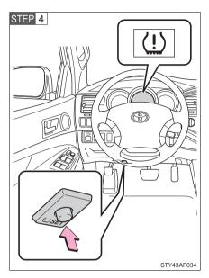
Push and hold the tire pressure warning reset switch about 3 seconds, and after releasing the switch the tire pressure warning light blinks slowly three times.
