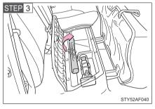
Unhook the strap and remove the tool bag.
