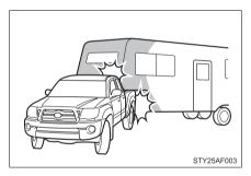
When towing a fifth wheel trailer, be careful not to hit the cabin or deck by the trailer while making a sharp turn.
