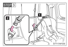
■ Route the top strap through the routing device as shown in the illustration.
