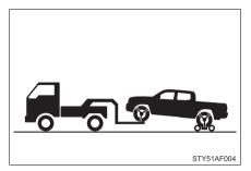
Vehicles with an automatic transmission: Use a towing dolly under the rear wheels.
