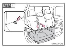
Swing the bottom cushion up by pulling the lock release strap.
