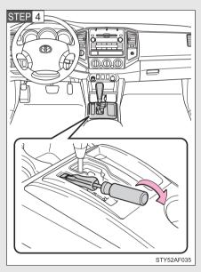
Pry the cover up with a flathead screwdriver or equivalent.
