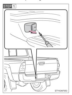
Remove the screw and light unit.
