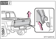
Tilt the tailgate to about 30° from vertical and pull up the right side of the tailgate to unhook the right side.
