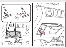
2.Pull up the box and disengage the claws. Remove the stoppers from the cutouts and remove the box. STEP 3 After a system failure, see "Fuse layout and amperage ratings" (→P. 396) for details about which fuse to check.
