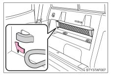
Cargo net hooks are designed to hang the factory-supplied cargo net.
