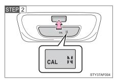
Press the switch until CAL appears on the display.
