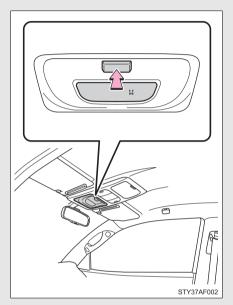
To turn the compass on or off, press the switch.
