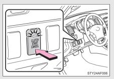
Press the CLUTCH START CANCEL switch to cancel the clutch start system when the engine switch is turned to the ON position.
