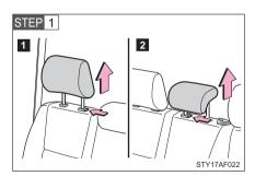
Remove the head restraint.
