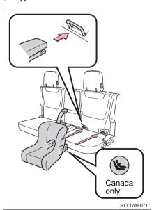
Latch the buckles onto the anchorages.
