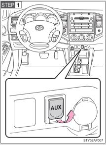
Connect the portable audio device.
