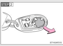
Remove the discharged transmitter battery.
