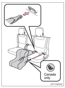
Latch the hooks of the lower straps onto the anchorages and tighten the lower straps.
