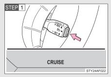
Press the ON-OFF button to turn the cruise control on.
