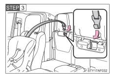
Latch the hook onto the anchor bracket and tighten the top strap.
