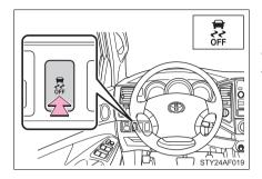
Push and hold the button for more than 3 seconds while the vehicle is stopped to turn off both TRAC and VSC.
