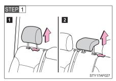
Remove the head restraint.
