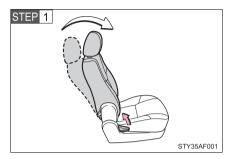
Pull the seatback angle adjusting lever and raise the seatback to its upright position.
