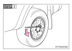
Slightly loosen the wheel nuts (one turn).
