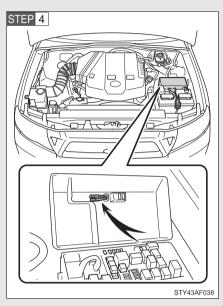
Remove the fuse with the pullout tool.
