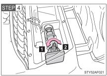
Loosen and remove the jack.
