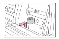
Remove the flashlight holder. It can be installed in various positions as required.
