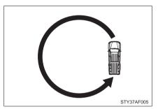
STEP 3 Drive the vehicle at 5 mph (8 km/h) or less in a circle until the direction is displayed.
