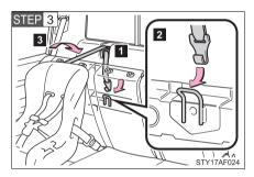
Swing the seatback forward slightly ( $\rightarrow$ P. 46) and remove the anchor bracket covers.
