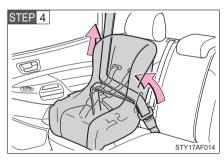
While pushing the child seat into the rear seat, allow the shoulder belt to retract until the child seat is securely in place.
